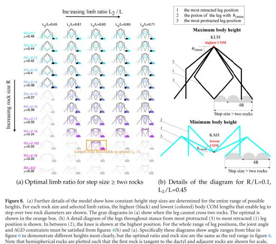
Note that hemispherical rocks are plotted such that the first rock is tangent to the dactyl and adjacent rocks are shown for scale, however, in stance the dactyl would be remain in the same valley while the COM moves horizontally so that the swinging leg move into position to the next valley. In other words, such diagrams are added to figure 7 with the dashed and solid lines showing most protracted and retracted postures, respectively.
