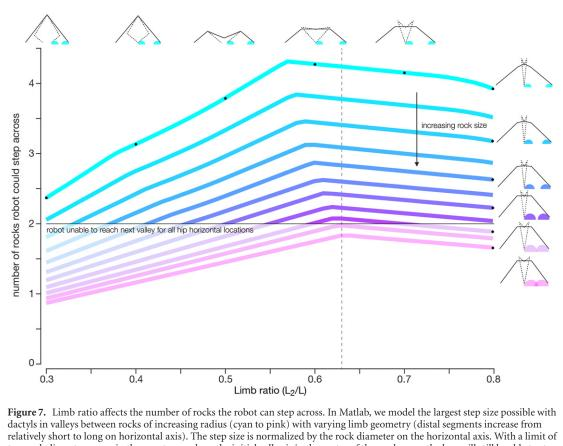
relatively short to long on horizontal axis). The step size is normalized by the rock diameter on the horizontal axis. With a limit of two rock diameters, even in the worst case where the initial valley is in the center of the workspace, the legs will still be able to step to the next valley while maintaining constant body height. Thus an optimal limb ratio of 0.63 (vertical dashed line) enables traversal of the largest rocks (maximum rock radius 18.5% of the leg length).
